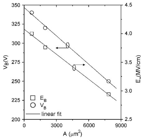
FIG. 5. Reverse breakdown voltage ( $V_B$ ) and breakdown field ( $E_B$ ) as functions of the device area  $A(=\pi d^2/4)$  for AlN APDs. The solid lines are the linear least square fits of data. The breakdown field of dislocation-free AlN epilayer ( $E_B$  at  $d=0$ ) is about 4.1 MV/cm.
